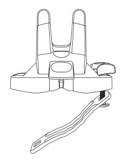
2. Position the base on the crossbar on the roof rack. Loosely install another bolt and knob as shown.
